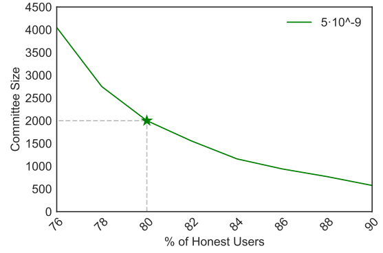
Figure 3: The committee size, \tau , sufficient to limit the probability of violating safety to 5 \times 10^{-9} . The x-axis specifies h , the weighted fraction of honest users. \star marks the parameters selected in our implementation.
